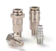
Safety coupling with UltaFlo-Valve for optimum flow and low pressure drop. The series stands out for its robust design (steel sleeve) and long service life even with the harshest use. Additional safety locking system. This safety lock prevents unintentional disconnection. To disconnect, the plug must first be pushed further into the coupling before it can be unlocked. The brass version has been developed specifically for use with water in the pressure range up to 35 bar.
